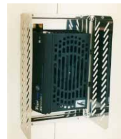
Rear view of incubator showing Tropicool unit; standoffs flat.
